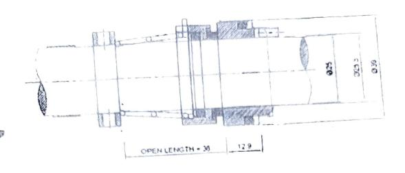
Rough Sketch for Item no. 4. Mechanical seal Lub oil pump ALEKTON Type- AH-240-800-2 GGSSTP material code 08050756
