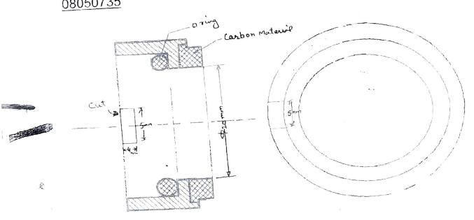
Rough Sketch for Item no. & Carbon ring with o ring For Lub oil pump ALEKTON Type- CF-240-800-2 ,GGSSTP material code 08050736
