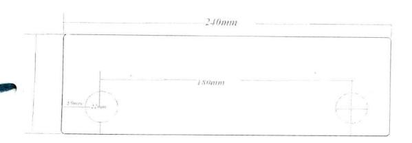
Lock Plate of size 240mm X 75mm X 25mm Material FE 410
