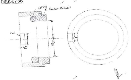
Rough Sketch for Item no. 3:- Mechanical seal Lub oil pump ALEKTON Type- CF-240-800-2 GGSSTP material code 08050752
